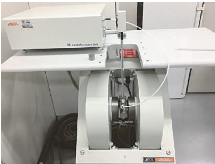
Figure 1 The electron spin resonance (ESR) / electron paramagnetic resonance (EPR) device for measurements of radicals in biosamples (JEOL JES FA-100).
