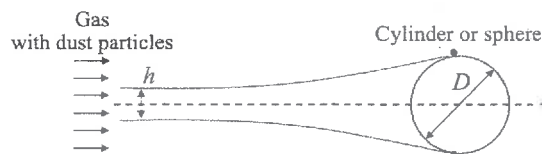
Figure Dust collection system
