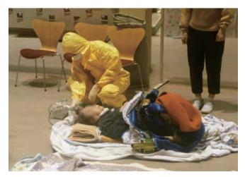
Radioactive contamination screening using GM survey meter
