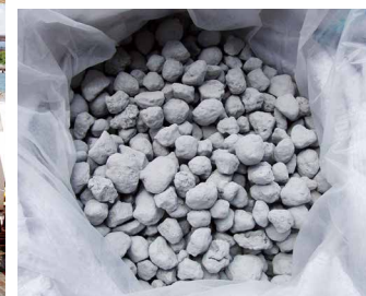
Granulated coal ash used to improve the sediment quality contaminated with organic matter
