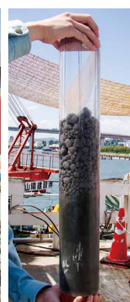
Sediment core sample collected from seabed after the improvement work
