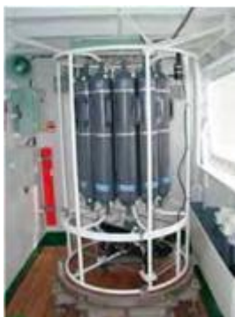
CTD 測定装置 (多筒採水器付) / CTD octopus system / and water sampling bottles
