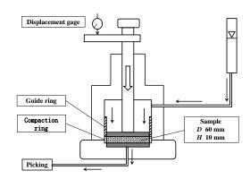
Fig.2 Consolidation and permeability testing apparatus
