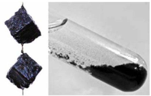
Fig. 1 Produced biogenic manganese oxide for adsorbing minor metals
